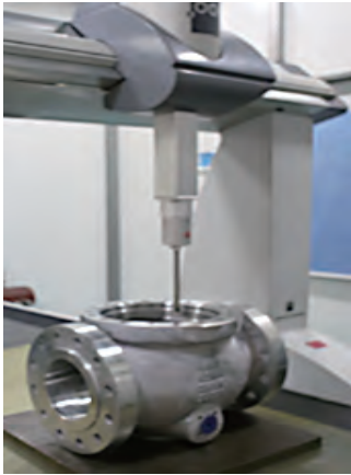
Three coordinate inspection of body
