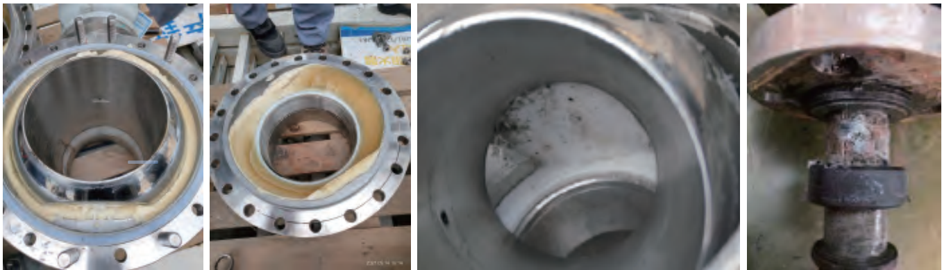
Ball valve blocked by medium solidification Ball valve blocked by medium self-aggregation Trunnion and bearing jammed by medium coking
