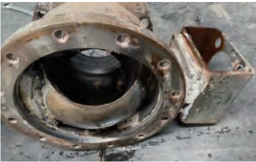
Coking in the valve body cavity
